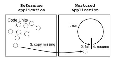
Figure 8.1: **Application tailoring with a run-fail-grow approach.** We (1) run the nurtured runtime and (2) detect the missing units on failure. For each failure, (3) we copy missing code units from the reference runtime and then (4) the execution is resumed (just before the failure point) until the process finishes.
