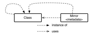
Figure 7.3: **Simplified Metatalk object model schema.** In Metatalk classes have no implicit metaclass. All classes share the same class. Mirrors are simple objects, thus instances of classes, that reflect on a class and contain their metadata. This schema does not represent the actual object graph, but a simplified picture.
