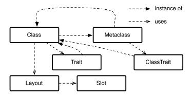
Figure 7.2: **Simplified Pharo object model schema.** In Pharo each class has a metaclass. Metaclasses are defined circularly. Both classes and metaclasses makes use of trait objects to define part of their behavior. Classes also have layout that includes first class instance variables (slots). This schema does not represent the actual object graph, but a simplified picture.
