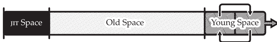
Figure 5.6: COG Memory Model Overview: Fixed-sized JIT space, slow changing old space and fast young space.
