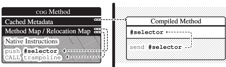
Figure 5.7: Cog Method: Compiled method representation at JIT -level residing in the JIT memory space.
