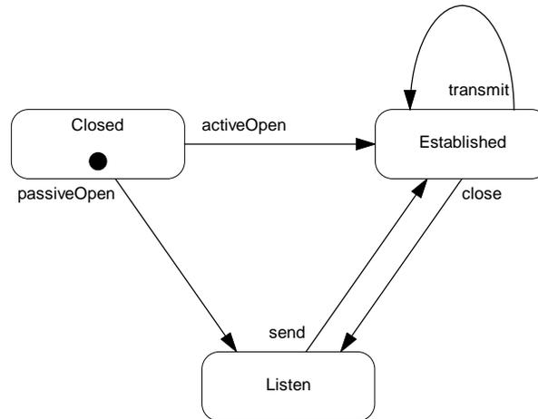
The TCPConnection begins its life in the Closed state. An activeOpen or a passiveOpen command will send it to the Established or Listen states respectively. Once in the Established state, a close command will send it to the Listen state, while a transmit command will perform an action, but keep it in the Established state. In the Listen state, a send command will transfer it to the Established state.
