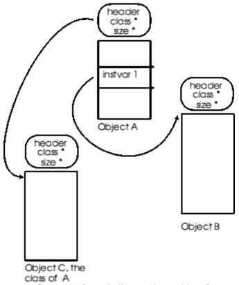
figure 11. Squeak direct pointer object format \* note variable object header format describe below
