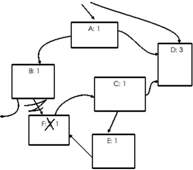
figure 5. Object B no longer points to F - the cycle F/C/E is orphaned
