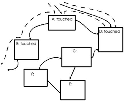
figure 6. Tracing objects in the mark phase
