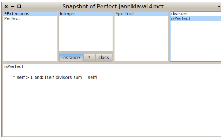
Figure 7.14: The snapshot browser reveals that the Perfect package extends the class Integer with 2 methods.
