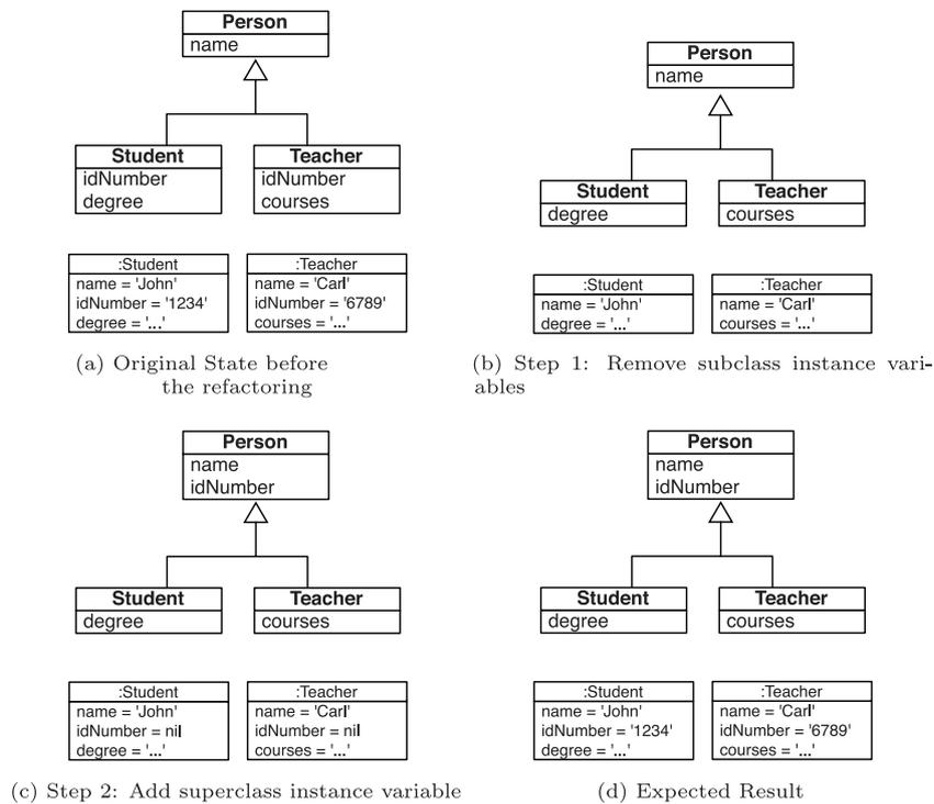
Fig. 1. Step by Step of applying the Pull Up Instance Variable refactoring to the *idNumber* instance variable present in *Student* and *Teacher* classes.
