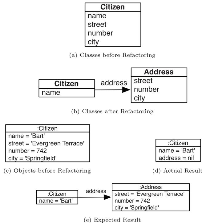
Fig. 2. The Split Class refactoring corrupts its instances.
