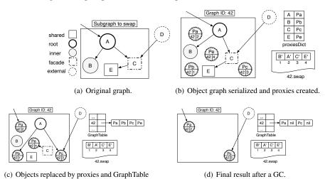
Figure 4 – Steps to swap out: Serialization, proxy creation, objects replacement and GC execution.
