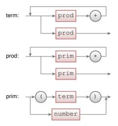
Figure 18.4: Syntax diagram representation for the term, prod, and prim parsers defined in script 18.15
