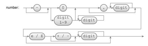
Figure 18.10: Syntax diagram representation for the JSON number parser defined in script 18.42
