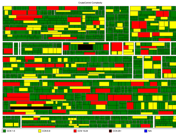
Figure 3.3: TREE MAP showing quality metrics in CruiseControl with methods as elementary boxes and classes as composed boxes.
