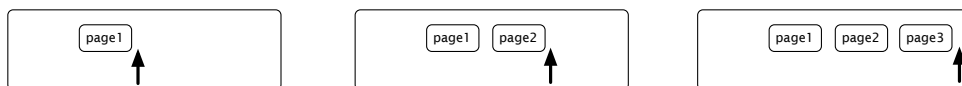
Fig. 5. A new history is empty. The user opens to page 1. — The user clicks on a link to page 2. — The user clicks on a link to page 3.
