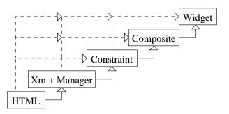
Figure 2. A concept inheritance hierarchy from the Mosaic system and X11 library in the "widget context". Dashed lines show the transitive closure of the inheritance relations.
