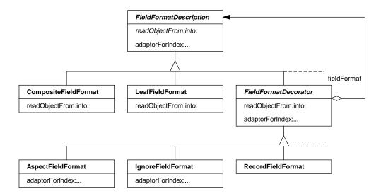
Let's look at how it's implemented. The superclass, FieldFormatDescription, declares the core interface for the entire hierarchy. It fulfills the role of the Component class. As an abstract class, it introduces basic messages like readObjectFrom:-into: and adaptorForIndex:andSubjectChannel:.
