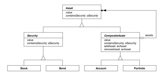
To implement this object model, first we'll implement Asset as the Component class. It does not need any variables. It declares two messages, value and contains-Security:, that its subclasses should implement.
