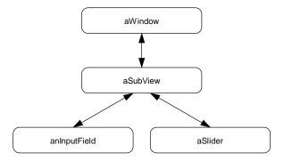
The three different kinds of nodes are easy to recognize by looking at how many components each one has. The window node has just one component. The widgets are leaf nodes because they have no components. The subview node is a branch node because it has multiple components. Subviews are the composite in the Composite pattern.
