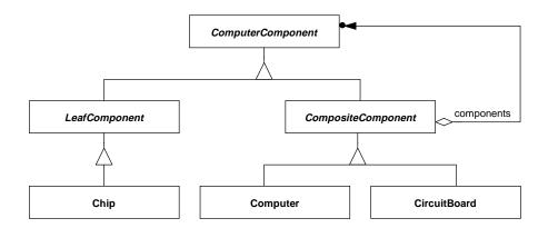
Chip is a Leaf class and Computer and CircuitBoard are Composite classes. The Composite class specifies that it can contain any Components, but its subclasses are more restrictive. A Computer can only contain CircuitBoards and a CircuitBoard can only contain Chips.
