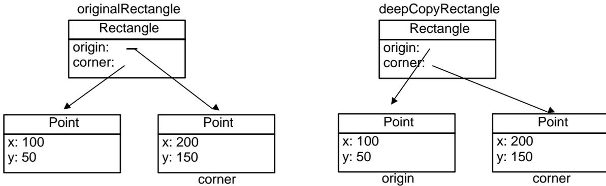
Figure 9.2. Shallow copy (top) and deep copy (bottom).
