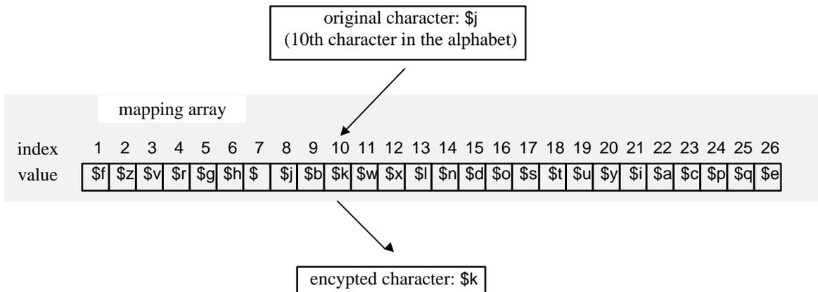
Figure 7.8. Encrypting secret message using a mapping array.
