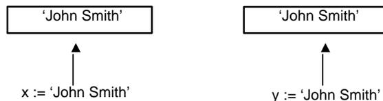
Figure 4.18. Two strings may be equal while not being equivalent.  $x=y$  is true but  $x==y$  is false.
