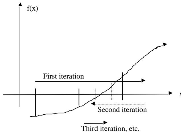
Figure 4.22. Finding root of  $f(x) = 0$  by iteration.
