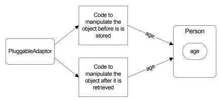
**Figure 24-9.** The PluggableAdaptor mechanism.
