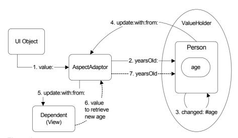
Figure 24-5. AspectAdaptors with a subject channel and different accessors.
