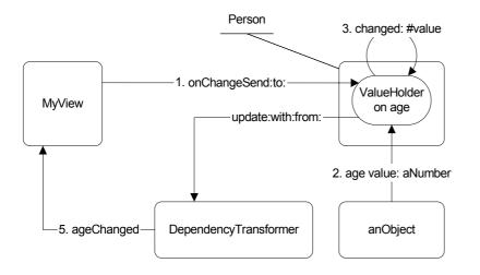
**Figure 24-3.** The ValueHolder mechanism.
