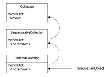
**Figure 2-1.** The method lookup mechanism.
