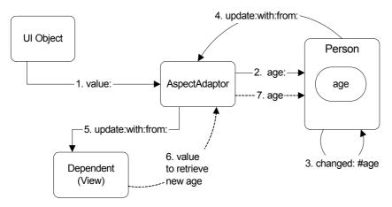
**Figure 24-4.** The AspectAdaptor mechanism.
