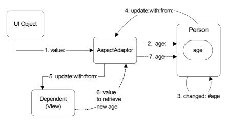
Figure 24-4. The AspectAdaptor mechanism.
